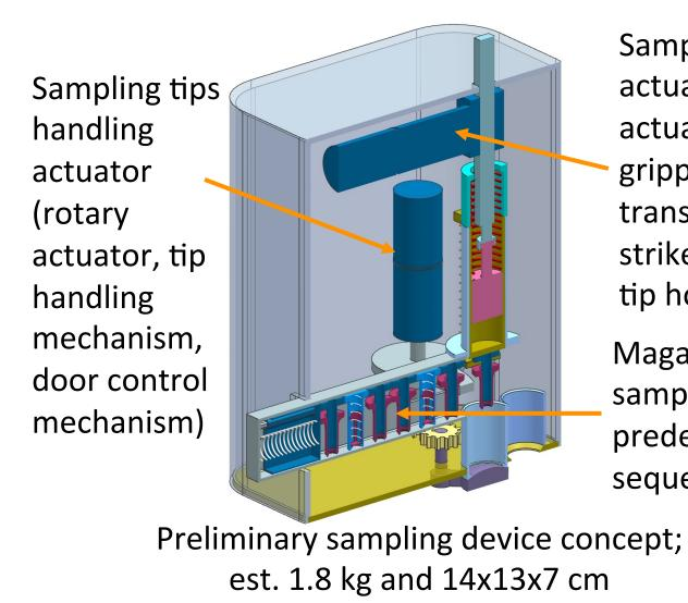
Sampling actuator (linear actuator, passive gripper, energy transfer spring, striker, sampling tip holder) Magazine with sampling tips in a predefined sequence)
